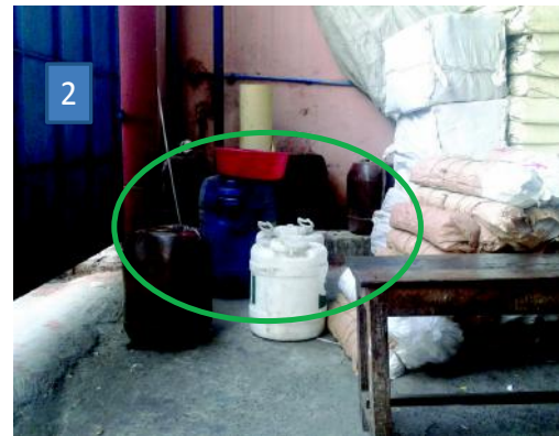
Diesel stored in cans near combustible material.
